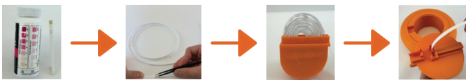
Strip dispenses out of the canister to be fed through the roller
